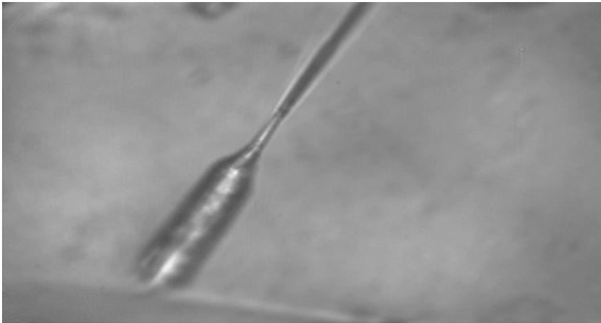
**Fig.1.** Track of high-energy galactic cosmic ray nucleus registered in the Marjalahti pallasite olivine crystal after 48 hour etching in WN solution. Photo size  $\sim (150 \times 300)$   $\mu\text{m}$ .
