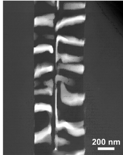
Fig.2. Dark-field TEM image of Ca,Cr-lamellae. Black and white platelets are diopside and chromite, correspondingly
