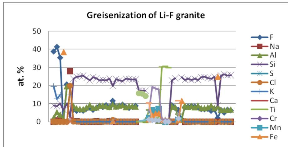
**Fig. 5.** Greisenization of Li-F granite, measured in 1 mm increments (open to the solution of the columns is at the left)
