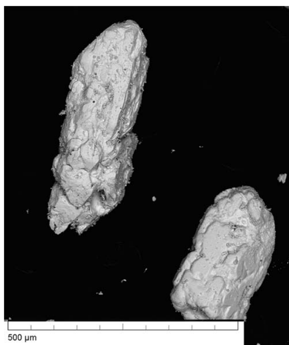
Fig. 4. Bismite crystals (photo by scanning electron microscopy)
