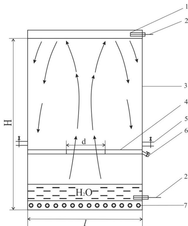
**Fig. 1.** The sketch of laboratory crystallizer for experiments to determine of mass vapor flow: 1 – condenser, 2 – thermocouples, 3 – crystallizer body, 4 – sampler, 5 – flanges, 6 – bibcock, 7 – electrical heater
