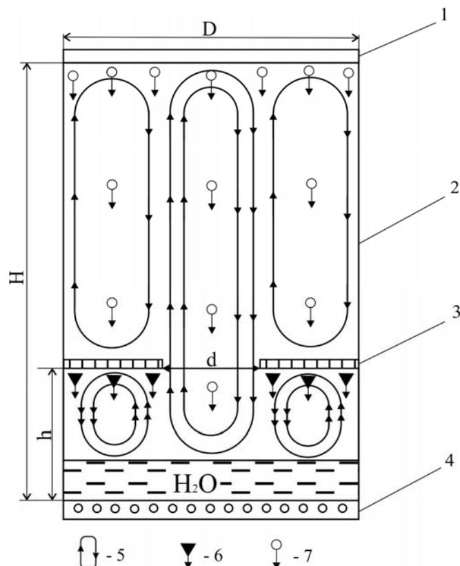
**Fig. 2.** The sketch of heat- mass transfer in crystallizer: 1 – crystallizer body, 2 – condenser, 3 – charge basket, 4 – electrical heater, 5 – free-convection cells, 6 – drops of condensate, 7 – drops of the solution formed in charge basket.
